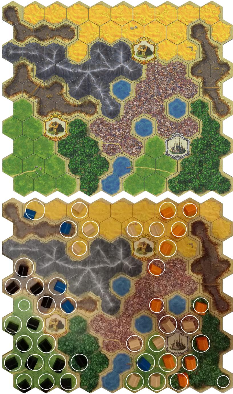
Figure 3.5: A scan of a board section (top) and an aligned board section from a photo (bottom) with hexes, in which a pair of SURF descriptors computed at identical locations in both images was found to significantly differ, labeled. The circle radii are proportional to the largest descriptor distance that occurred within a hex.
